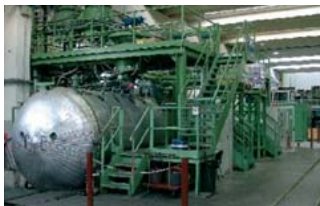
^ The pouring system under high vacuum
