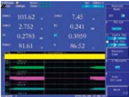
< Current pulses consumed by induction heating
